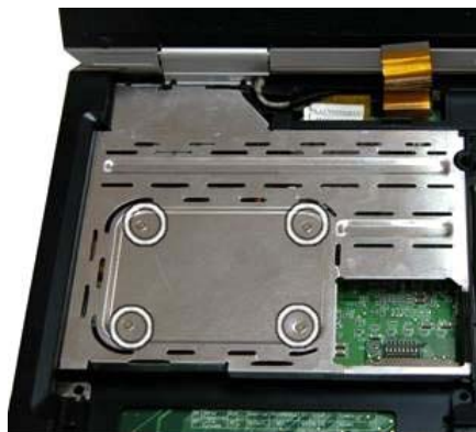
Fig. 17 Removing the heat plate screws
